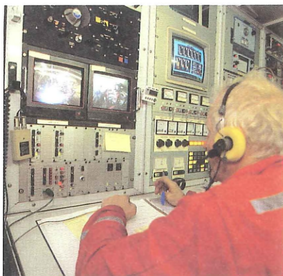
Welding supervisor Dave Savage of the "Pelican" guiding the welding robot from the control centre on board the vessel. The weld is made in 70 metres of water depth within a special seabed habitat.
