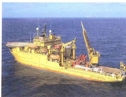
"Seaway Pelican" was responsible for changeover of three gas pipelines: to Emden, Gyda and Tor. Work on the 36 inch Emden export line took almost seven days. On the two smaller lines completion came sooner, taking less than five days.
