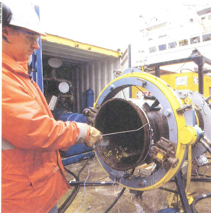
The pipe-cutter undergoing tests before getting to grips with the 24 inch Eldfisk crude line. Derek Usher on "Semi 2".
