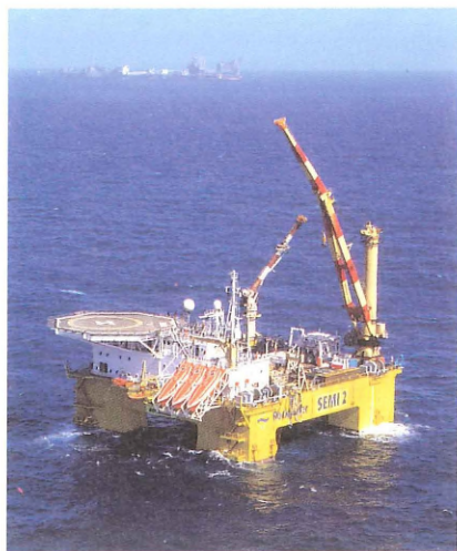
"Rockwater Semi 2" commenced by connecting up the oil pipeline from Valhall to Ekofisk II, a job that took seven days. Then followed the Eldfisk oil line (nearly six days), and the Eldfisk gas line (six days plus).
