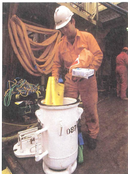
Lasse Tveit "feeding" the "Pelican" divers through the pressure hatch.
