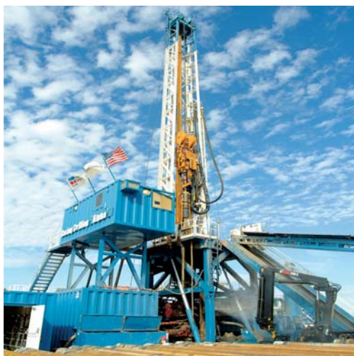
Casing drilling in operation at Lobo field, south Texas.
